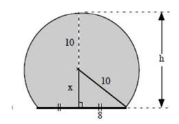
the diameter drawn is the perpendicular bisector of the chord:  $\Delta$  is right-angled so can apply Pyth. Thm.
